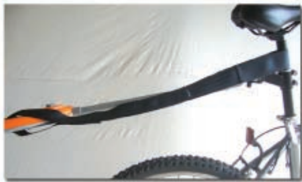
Safety strap, make sure that it is secured at each end.
